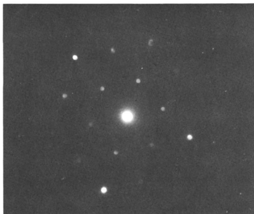
Figure 11. Anomalous diffraction pattern of a small metallic particle, showing 2.46 Å spots.
